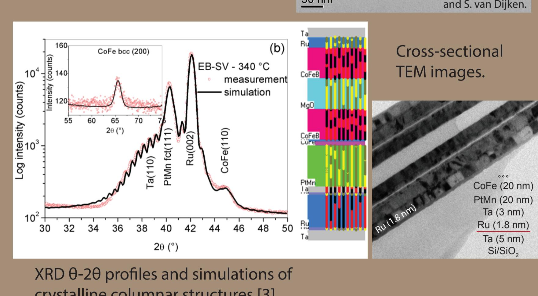
XRD  $\theta$ - $2\theta$  profiles and simulations of crystalline columnar structures [3].
